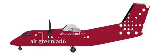
Quantity: 8 Max. no. of seats: 37 Average speed in km/h: 537 Max flying altitude in m: 7,620
